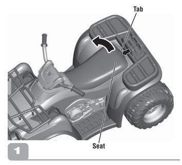
· Press the tab on the rear of the seat and lift to remove.
